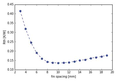
Figure 3. Heat sinks calculated with different fin spacings
