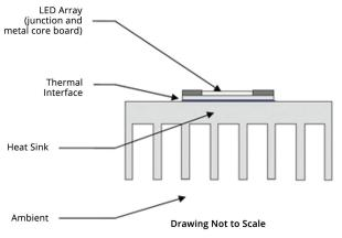
Figure 1. Typical setup of thermal resistance
