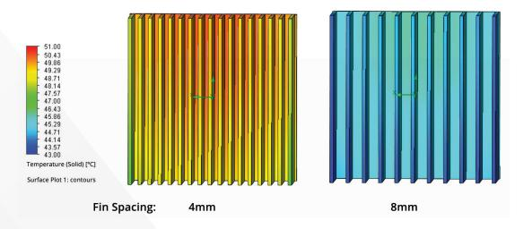
Figure 4. Optimum fin spacings of approximately 6-10mm free space
